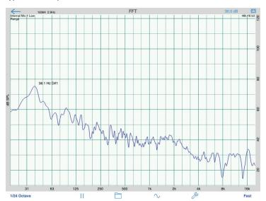
This FFT graph shows the Sound Pressure Level across the audio frequency band 20 Hz to 20 kHz, after the Fast Fourier Transform has been applied mathematically to the microphone measurements.
