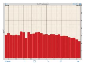
This graph shows the Sound Pressure Level measured by the microphone across the audio frequency band from 20 Hz to 20 kHz. In this example, the measured response starts to decrease at the higher frequencies.
