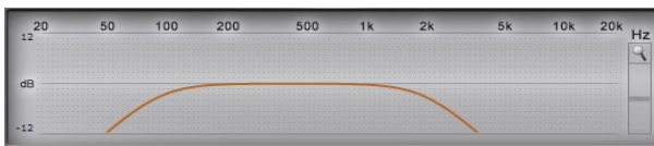
Crossover frequency 80 - 2000 Hz @ 12 dB/Oct.
