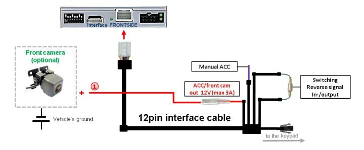
1 The red power supply output ACC/front cam out 12V (max 3A) can be used to power a front camera. If Dip 1 is set to ON (black 8 dips), the power supply output gives +12V (max 3A) when reverse gear is engaged incl. 10 seconds delay after reverse gear is disengaged.
