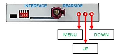
The picture settings are adjusted by the 3 buttons on the video-interface. Press the MENU button to open the OSD settings menu. To switch to the next menu item, pressing UP and DOWN will change the selected value. The buttons are embedded in the housing to avoid accidental changes during or after installation. The picture settings have to be done separately for AV1, AV2 and CAM while the corresponding input is selected and visible on the monitor.
