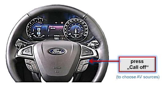
Switching the video sources can be done by a long press of the vehicle's **Call-Off button**
