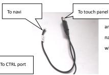
The CTRL port can be connected to the left touch cable, so DVD and other devices can be touch controlled. The internal switch makes the navi use touch panel when in RGB-input, and DVD uses the touch panel when in AV1 input.
