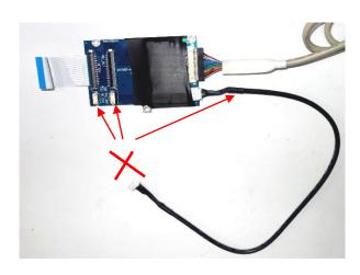
These 3 connectors pointed by red arrow should be **NOT** connected [also no connector to wire to.].
