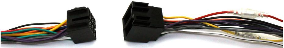
7. Connect the female vehicle specific connectors on the harness to the male vehicle connector from the vehicle. Test head unit for correct operation.
