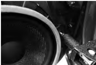
Assemble the Focal speaker using the rivets provided with the kit IS 165TOY
