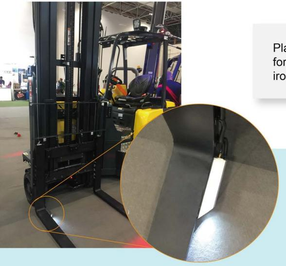
Place the magnetic base forklift camera on the iron arm.
