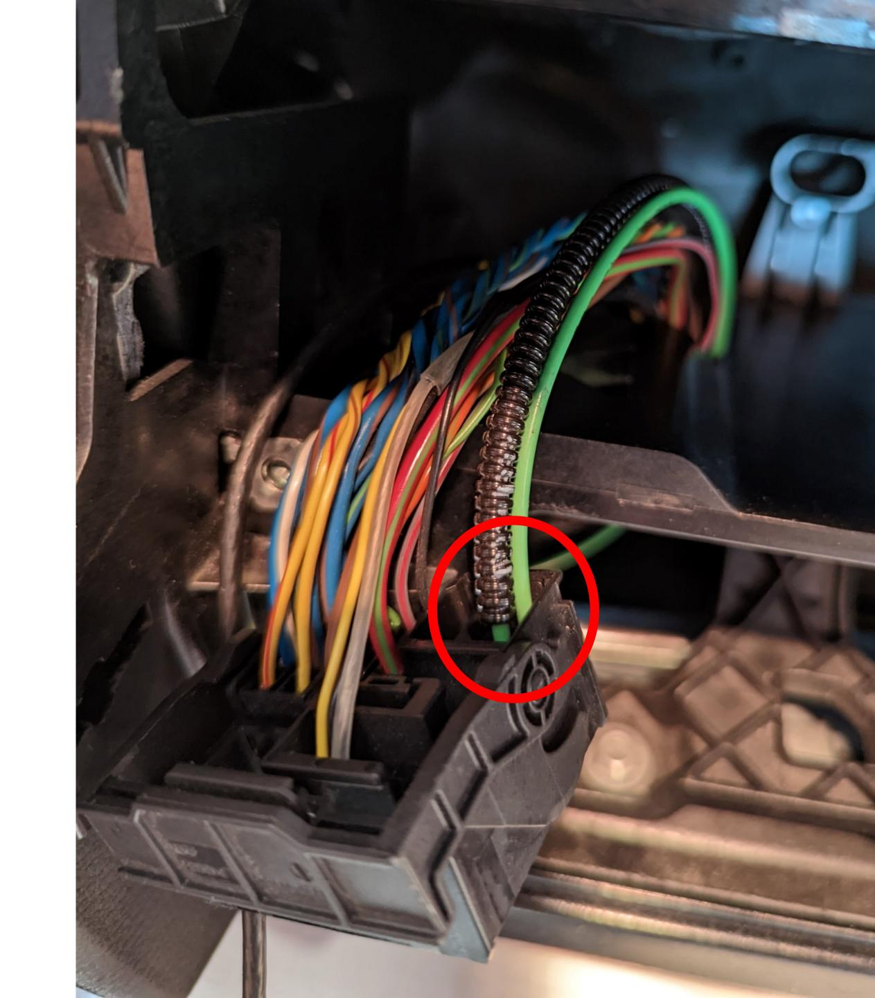
Under the fiber optical cable the is a little lock. Use a small flat screwdriver or something tiny to loosen the connector.
