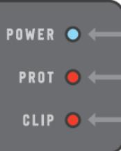
**POWER (blue LED):** Indicates that the amplifier is on when it is on.
