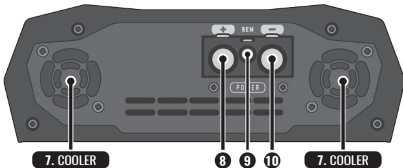
**7. COOLER:** It cools the amplifier. Install in a cool place being careful to not obstruct the air vents.
